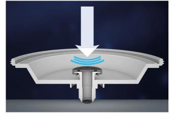
Oscillating non return valve ensures that the non return valve is not blocked with any dirt.
