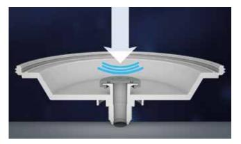
Oscillating non return valve, makes sure that the non return valve can not be blocked from any dirty.
