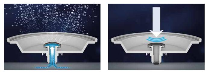
Oscillating non return valve, makes sure that the non return valve can not be blocked from any dirty.
