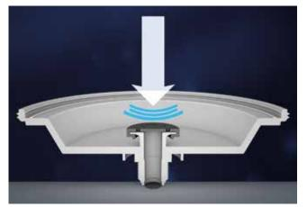
Oscillating non return valve, makes sure that the non return valve can not be blocked from any dirty.
